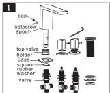
1.To Separate the spout/hadle sets from vavle sets by allen key orderly as drawing.
