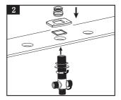
2.Make sure there are four holes in your table. Put the washer into the groove of base, put the base on the hole and adjust the position correcty, use the top valve nut to tighten the valve body, tighten the valve with locknut of the valve bottom.
