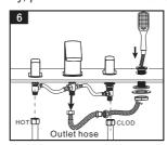
7. tigten the hand shower on the shower hose, the shower hose pass the hole on deck, and connect with the outlet on the valve. Installation steps, check every joint to ensure it has been connected well.
