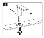
3.Install the spout through the middle hole to the connector of valve, lock it by the screw and put the cover to the screw hole.
