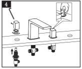
4.Install the handle valves to the hole from the bottom to the top, tighen with base from the top and tighten it with fixing part undemeath. Put the handle to the cartridge spindles, locked with screw by allen key, put the cover to the screw hole
